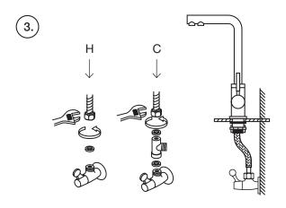
Now connect the hoses for hot and cold water, colored red and blue respectively. Connect the cold on top of the T-fitting, as pictured.
