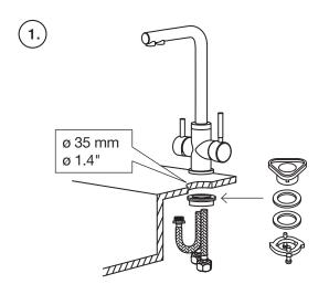
Before installation, make sure the surface hole is  $\emptyset$  35 mm, that the bottom rings are dismantled and that the hoses are connected to the faucet.
