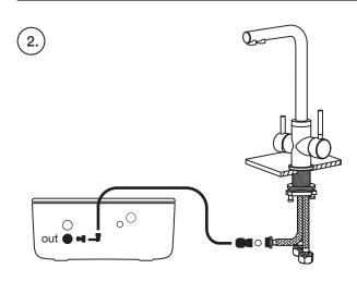
See "Outlet circuit installation" in the water purifiers installation guide to connect the purified water. Use the straight female connector that comes with the faucet.
